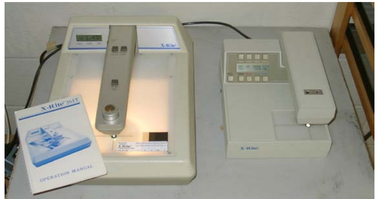
Figure D.7 X-Rite Model 361T (left) and Model 820TR (right) densitometers used for reading all negatives.
